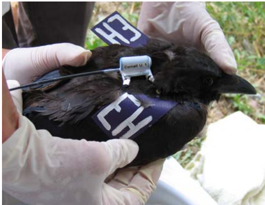
Fig. 4 American Crow with prototype DSSS transmitter
