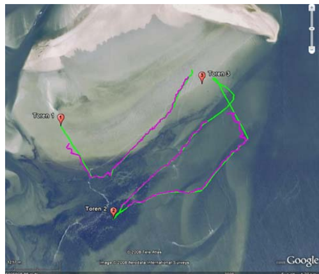
Fig 9. Boat track in Wadden Sea comparing Automatic System and GPS
