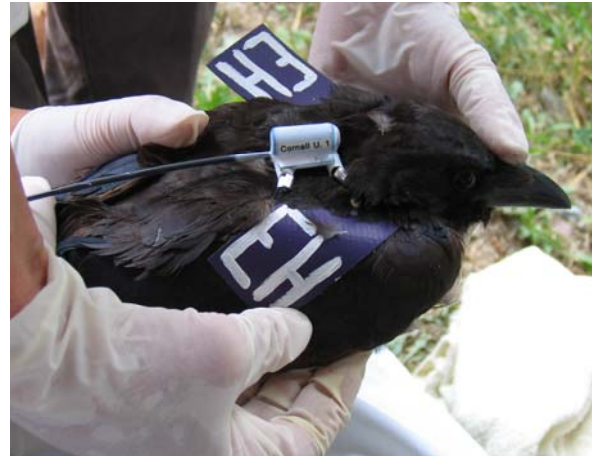
Fig. 7 American Crow with prototype DSSS transmitter
