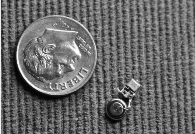
Figure 33.2 A 110-mg tag, adapted from Reference 40, built by Julian Kapoor at Cornell University.
