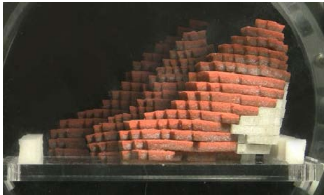
Fig. 4: A time-series example of a fabricated soft robot, which actuates with cyclic 20% volumetric actuation in a pressure chamber (J. D. Hiller and H. Lipson 2012). This proof-of-concept shows that evolved, soft-bodied robots can be physically realized. Current work is investigating soft robot actuation outside of a pressure chamber.
