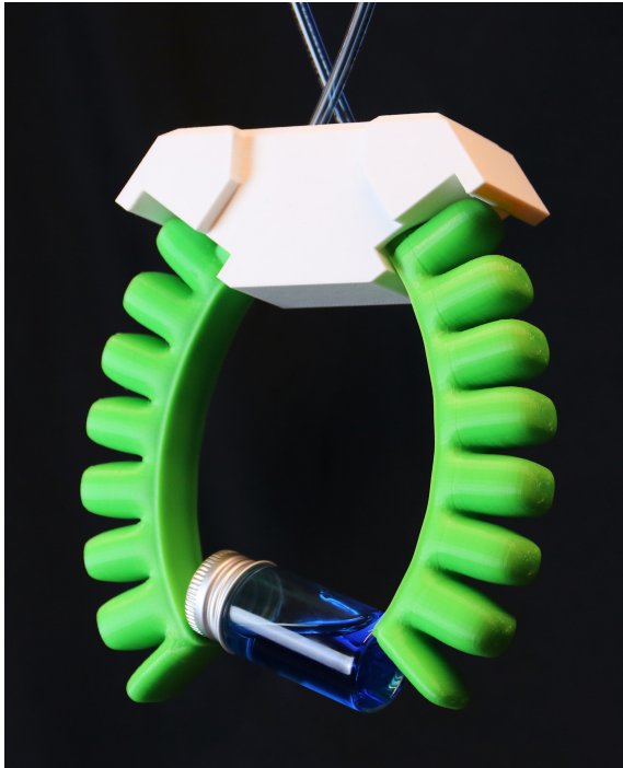
Fig. 7: Soft gripper capable of grasping delicate objects, designed, characterized, and fabricated using the workflow described in this paper.
