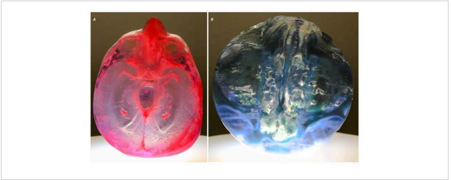
Figure 5: Potential problems. Two images of two different models demonstrate the issues around the clarity of working with translucent materials. (A) This model shows the result of enclosed voids within the model that have been filled with a 'support' material by the printer. In this model, the voids were intentionally created to create a variation in optical properties. (B) This model shows open voids that run deep into the model. The voids are tortuous, making standard postprocessing techniques, which polish the surface, impossible. The resulting optical distortion has rendered the model unusable for clinical applications. Please click here to view a larger version of this figure.
