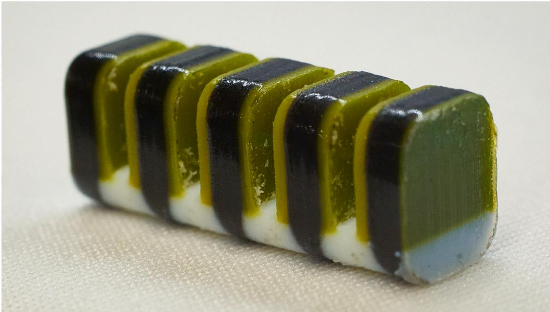
Fig. 7. Soft actuator printed in three materials. This example was created using a scalar field equation in polar coordinates with a threshold of 1 to generate the geometry, and was then functionally graded in threshold mode using three distinct scalar fields over the entire bounding box of the model. The above image is the resulting model, printed using the Stratasys J750 InkJet Printer. The OpenVCAD script for this object is provided in Fig. A.19.
