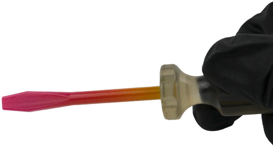
**Fig. 14.** The screwdriver from 13 (b) constructed using a Stratasys J750 Polyjet printer. Multiple materials are used to add a soft-touch handle and a multi-color shaft. (For interpretation of the references to color in this figure legend, the reader is referred to the web version of this article.)
