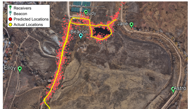
Figure 1. Field testing results overlaid on a satellite photo of the test site. The yellow line shows ground-truth GPS measurements while the red dots are positions calculated with our time-of-arrival system. The RMS difference between our system and GPS is approximately 22.6 meters.
