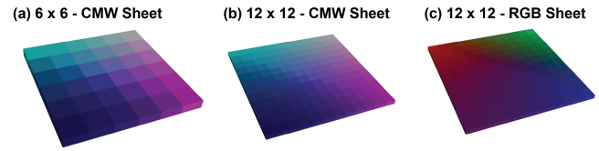
Figure 2: Color calibration sheets created using pyvcad. (a) 6×6 grid using cyan, magenta, and white (CMW). (b) 12×12 CMW sheet. (c) 12×12 grid with red, green, and blue.
