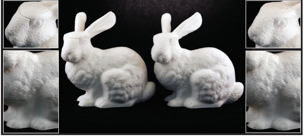
Figure 10: Printed fuzzy-skin bunnies compiled from semantic setting fields. The unblended bunny has sharp texture transitions at semantic-region boundaries, while the blended bunny uses a joint 12 \times 12 settings partition to produce smoother texture variation.
